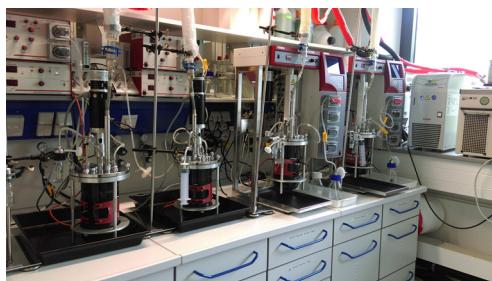
Fig. 5. Bioleaching for metal recovery in stirred reactors in the BGR geomicrobiology laboratory.
